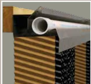
The **CLOSED TOP SYSTEM** is extruded from ultraviolet stabilized PVC for durability and ease of installation. The hinge-open cover and thumbscrews allows accessibility to the spray bar and hold pads firmly in place. The spray bar bracket and water deflector insure pads are uniformly wet.
