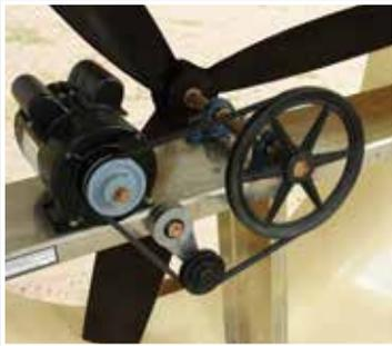
composite fiberglass and engineered with a true airfoil design that increases the overall efficiency of the fan. Drive shafts of 1" material allow for large, cast iron, greasable pillow block bearings to be used for longer life. Large pulleys allow for longer belt life and smooth operation.
