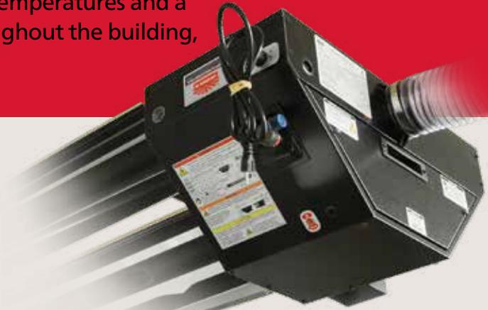
The AV2 Series upper combustion tubes contain the flame and operate at higher temperatures. Each tube has its own reflector allowing the hotter upper combustion tubes to concentrate more energy to the perimeter of the heating pattern.
