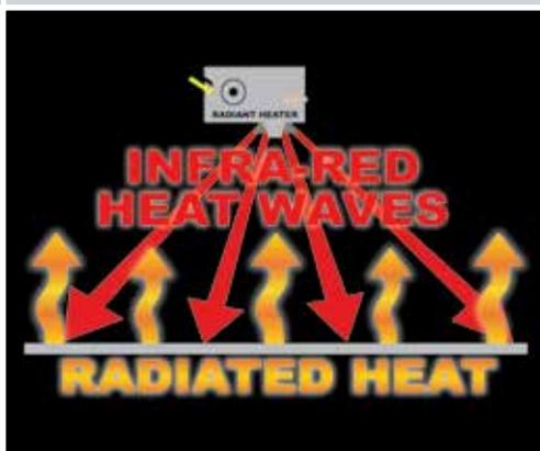
Infra-red heat emulates the true efficiency of the sun. It generates energy that is converted into heat when absorbed by objects like floors and animals. The energy is then re-radiated to warm the surrounding area by convection. This is the most efficient method of heating many poultry facilities.
