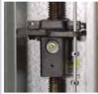
The drive block assembly features a removable nylon insert in a heavy-duty cast iron drive block simplifying cable/chain installation and ease of maintenance. This design also decreases friction and provides wear characteristics superior to conventional brass drive blocks. UHMW polyethylene guide wheels insure smooth travel, proper alignment and stability.
