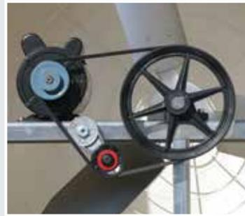
Features include a 1.5 HP single phase motor or a 1.75 HP three phase motor, easy belt access, fiberglass housing and cone, and stainless steel hardware. The belt driven 54" competitor series fans feature an automatic belt tensioner for smooth operation. Like all Cumberland belt drive fiberglass fans, cast iron pulleys and greasable pillow block bearings are standard features.
